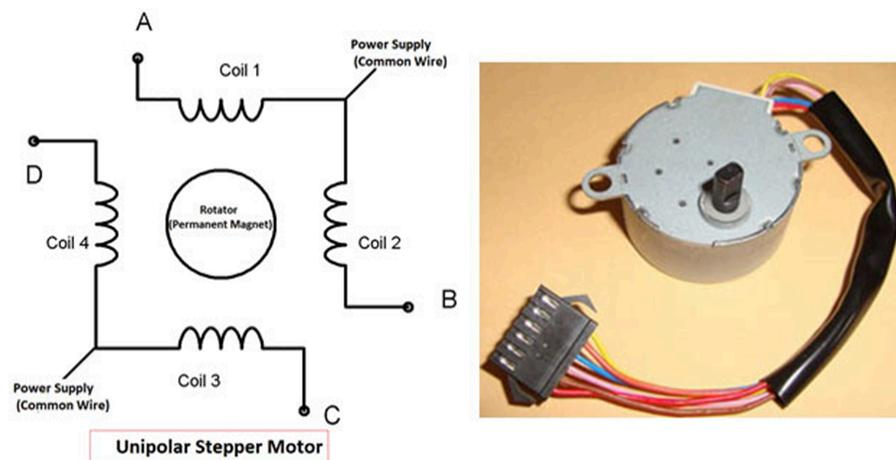
triggers, we control the power pulses and hence the speed of the stepper motor.
