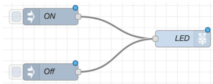
With that done, we have now completed our very first Node-Red Flow. Next step is for us to **deploy the flow on the raspberry pi**. Click the red deploy button. You should see “successfully deployed” flash at the top of the screen as shown below.
