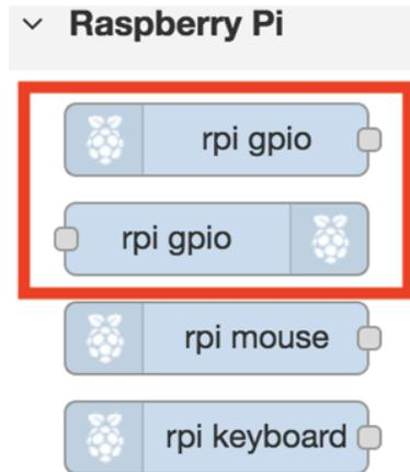
To begin, Scroll to the bottom of the Nodes palette, you will see the raspberry pi nodes section towards the end with two nodes labeled **rpi gpio**. These nodes are used for communicating with the raspberry pi's GPIO. One of the Nodes is for input while the other is for output differentiated by the position of the raspberry pi's logo. For the **input node**, the logo comes before the text, while for the output **node** the logo comes after the text as shown in the image below.
