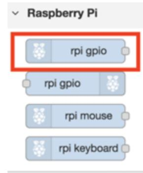
Drag the node into the flow and double click on it to edit properties. Set the pin to GPIO 4 (pin 11) and set the dropdown in front of the resistor to pull-up. This will “pull up” GPIO 4 to HIGH. Click on the done button after setting the properties.
