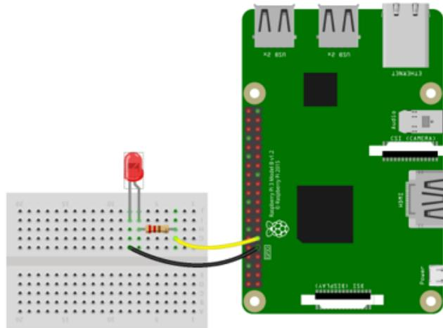
I also build the same on my hardware using a breadboard, LED, resistor and some connecting wires. My hardware set-up looks something like this once the connections are made.
