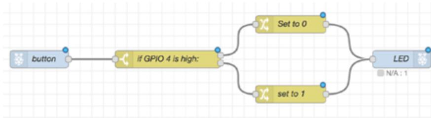
successful you should see the deploy successful popup and now be able to control the led using the switch.
