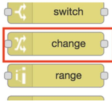
We will be using two of the change nodes. The payload of the first one will be set to 0 as shown in the image below and the payload of the second one set to one. Click done after editing properties for both.
