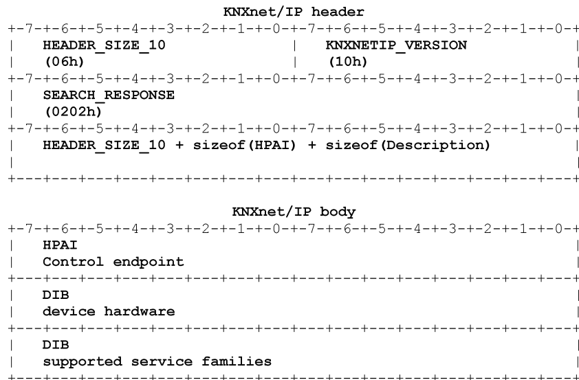
Figure 20 — SEARCH_RESPONSE frame binary format
